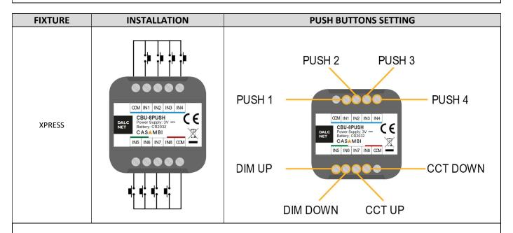
With this fixture it is possible to setting up to 4 N.O. push buttons. Each push button can control a luminaire, control a group of luminaires, control a scene or an animation, SAME FUNCTIONS AS IN "4 in" Fixture. This configuration is possible to set by Casambi APP.
