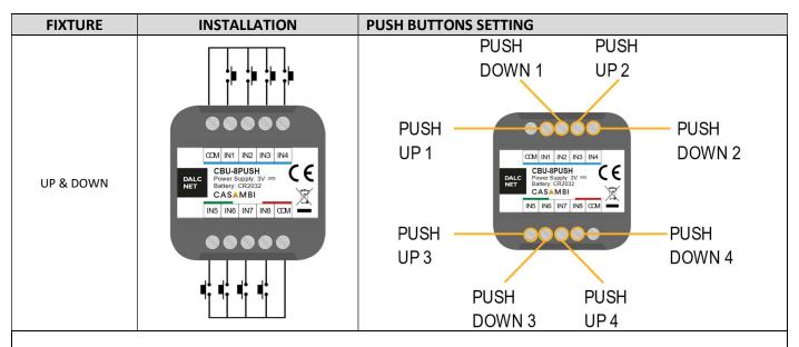
With this fixture it is possible to set 4 couples of N.O. push buttons, where each couple has got one button for dimming UP luminaire and one for dimming Down. In total there can be connected 8 N.O. push buttons.
