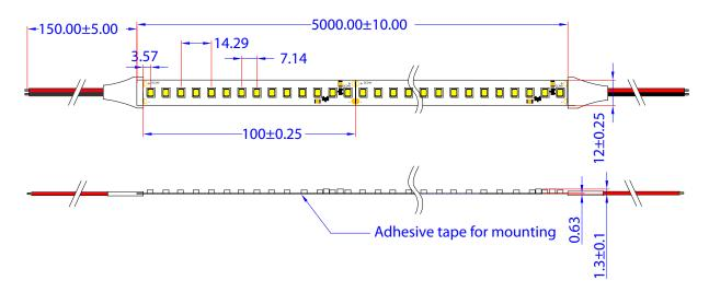
Notes: 1. All dimensions are in millimeters. 2. Tolerance is ±0.20 mm.
